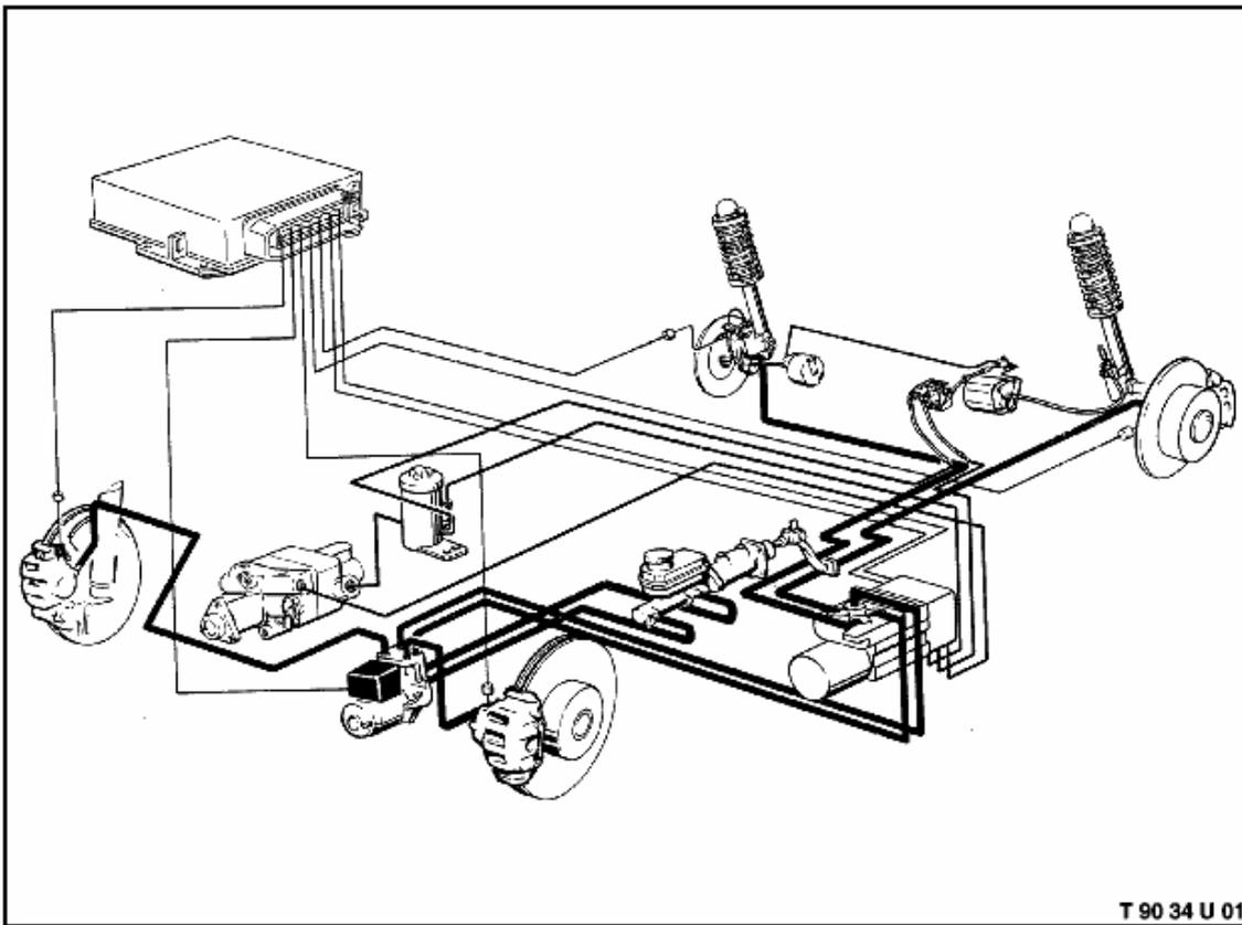
The same principle is applied to wheel slip when accelerating (wheel spin) by the ASC system. By controlling throttle opening and ignition timing, ASC reduces torque to the driven wheel if excessive wheel slip occurs during acceleration. More effective transmission of power to the road surface is achieved, and lateral locating forces remain high (resulting in greater vehicle stability).
