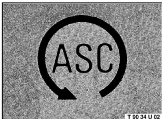
Whenever the ignition is switched ON, the ASC+T system is in operation. The indicator lamp goes off when the engine is started. As soon as the system is **activated**, for example, if the accelerator setting is excessive for the given road conditions, the ASC lamp in the instrument cluster flashes to alert the driver. If the ASC+T system fails or is switched off, the ASC lamp remains ON permanently.
